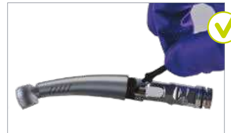
Replacing a water filter
