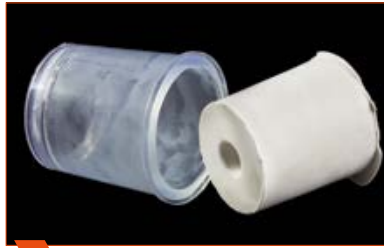
2 Press the investment ring carefully out of the silicon ring.
