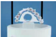
Correct position on the sintering tray
